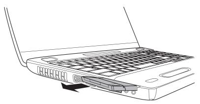
Figure 8-2 Removing the PC Card
